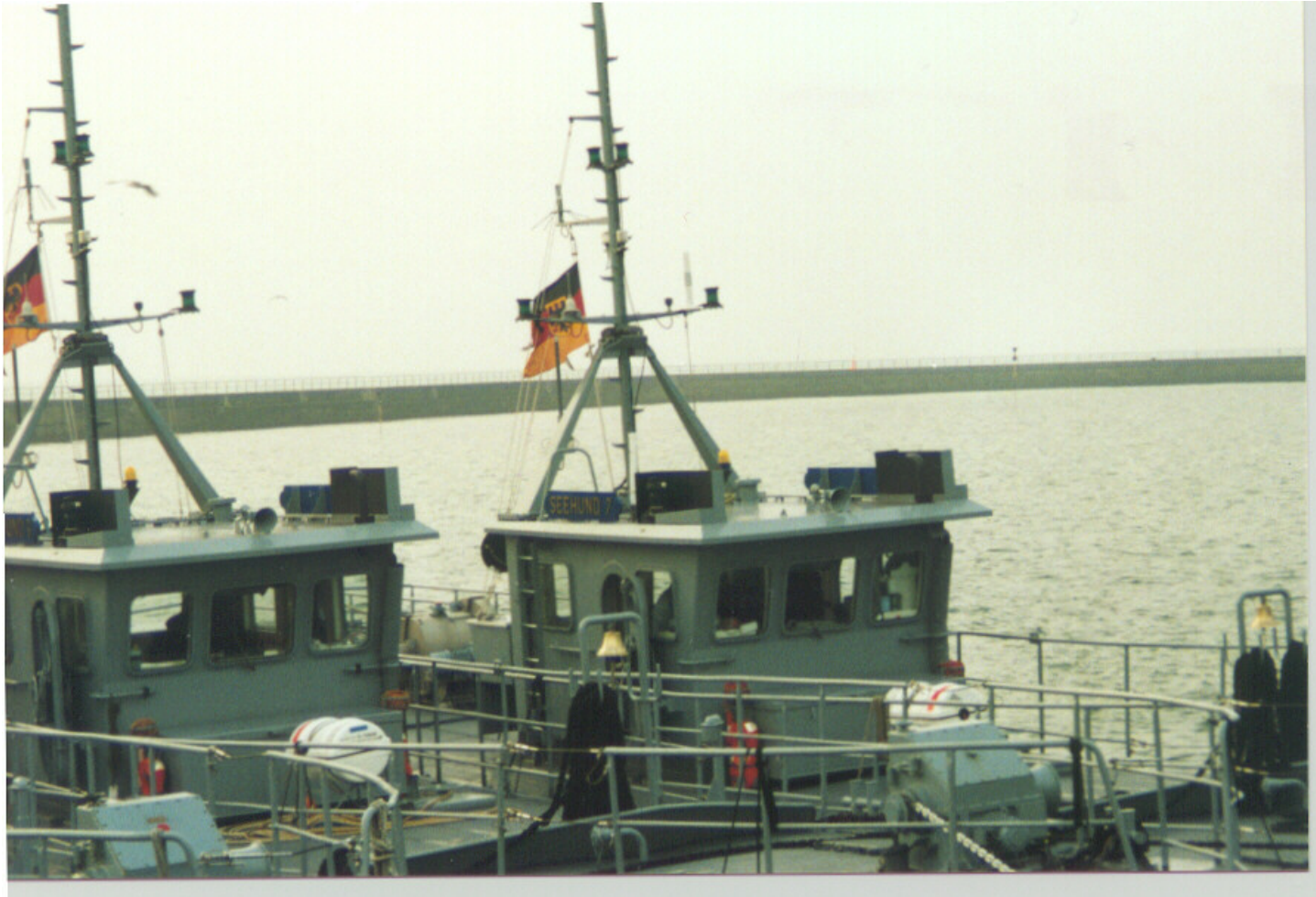
Drone vessel Seehund 7 with SatMate Receiver
