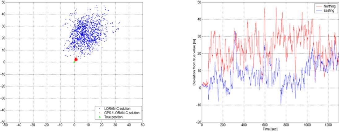
Figure 6: Left: Position fixes from Loran-C after a calibration phase, right: Time series of respective north and east coordinates.
