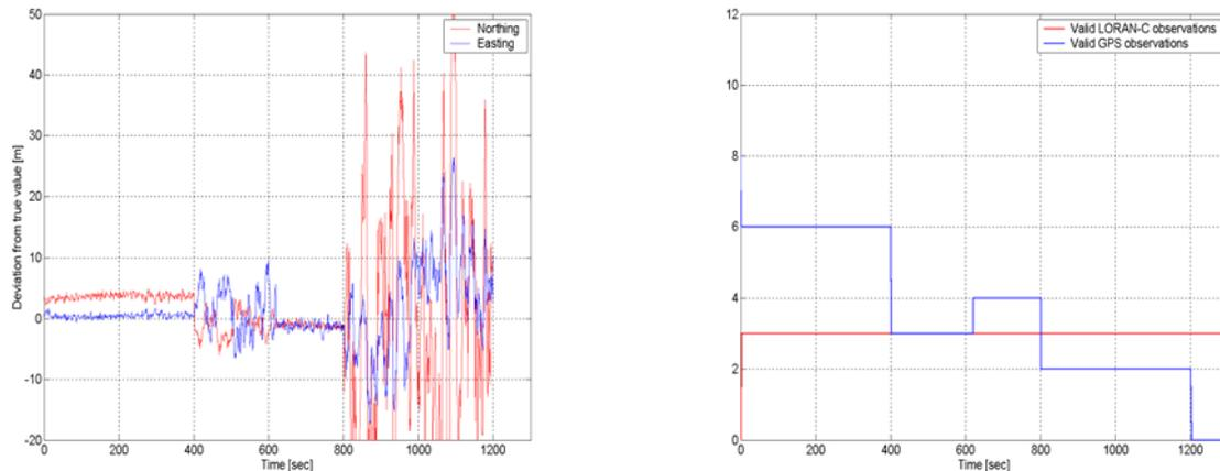
*Figure 8: Left: Position fixes from an integrated GPS/Loran-C solution under changing satellite visibility, right: Number of visible navigation sources.*
