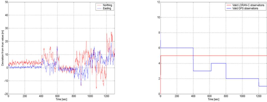
Figure 7: Left: Position fixes from an integrated GPS/Loran-C solution under changing satellite visibility, right: Number of visible navigation sources.
