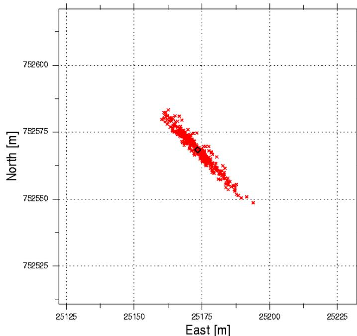
*Figure 3: Scatter plot of Loran-C position fixes (Gauss-Krueger projection). The repeatable accuracy is about 13 m (95%) in north and east direction. The across error is only about 5 m (!).*
