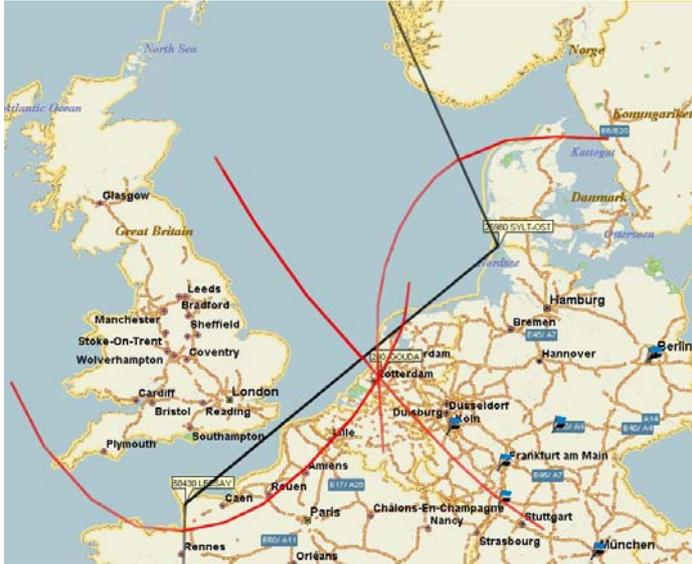
Figure 4: Geometric situation at the measurement site in The Netherlands. The red curves represent the Loran-C hyperbolas for the TDs between the transmitter stations at Lessay and Sylt (low curvature hyperbola at the center of the figure), Lessay and Soustons (bottom left), and Sylt and Værlandet (top right).
