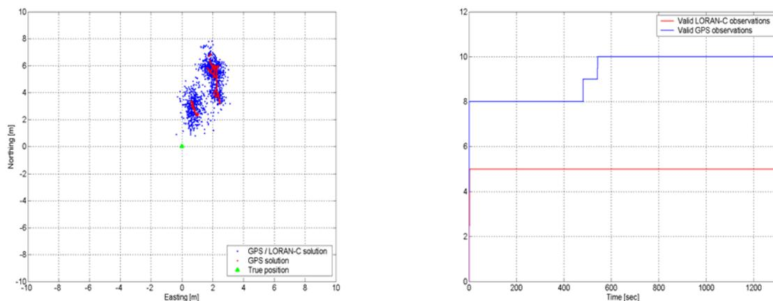
Figure 5: Left: Position fixes computed from all GPS stand-alone and integrated GPS/Loran-C, right: Number of visible navigation sources.
