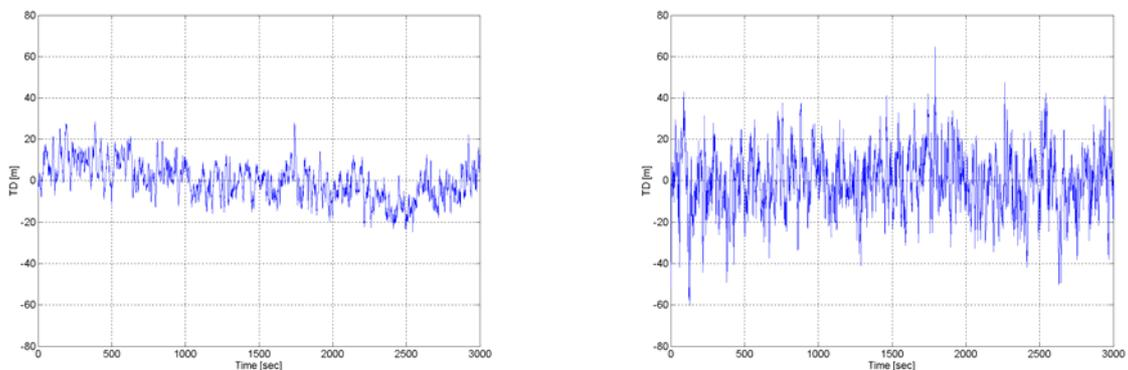
Figure 2: Differences of TOA time series (left: Chayka: 8000M – 80002, right: NELS: 6731M – 6731Z). Note: The unit of the vertical axis is meters.
