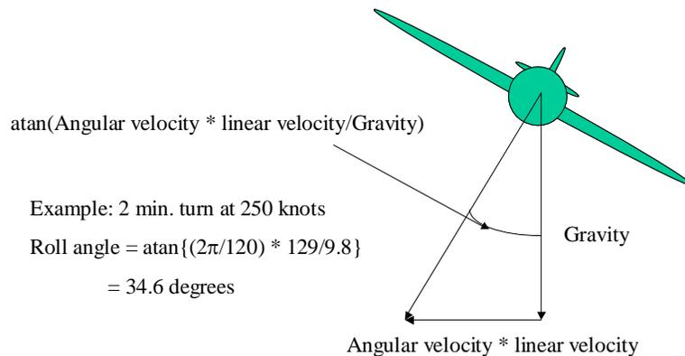
Figure 5. Estimation of roll angle from position data.
