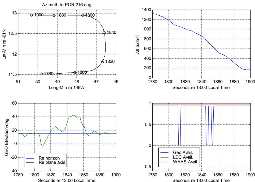
Figure 7. Geo elevation and WAAS message availability during landing at Merrill Field, Ohio U. King Air on August.24<sup>th</sup>.
