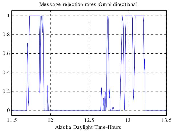
Figure 14. Message rejection rates for Ohio University August 24<sup>th</sup> flight using an electric field antenna.
