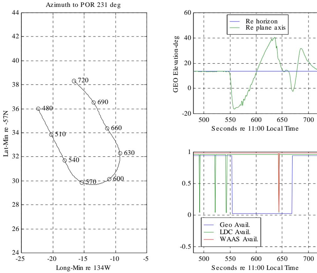
Figure 6. Example geo elevation calculation and WAAS message availability during turn south of Juneau Convair 580 on August 23<sup>rd</sup>, speed over ground 300kts, distance to Tok 423 nm.
