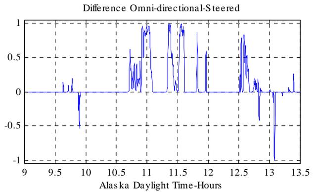
Figure 9. Byte error rates for Convair 580 and Tok transmitter peak power for August 23<sup>rd</sup>.
