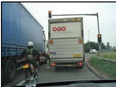
Figure 6: Lorries in the M1 Motorway blocked GPS signals and potentially caused dynamic multipath.
