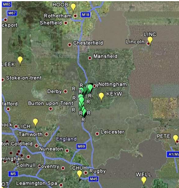
Figure 2: SmartNet CORS configuration used during both tests (icons in yellow, HOOB, LINC, LEEK, LICH, CHUK, WELL, PETE and KEYW). Vehicle route is indicated in green. The average distance between CORS is about 47.32 km.
