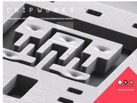
Figure 3 – Inside of a MEMS yaw-rate sensor.
