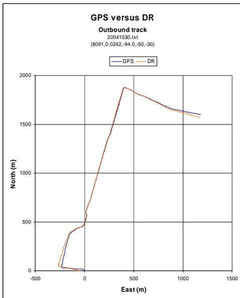
Figure 1 – Estimated and true track of test runs.
