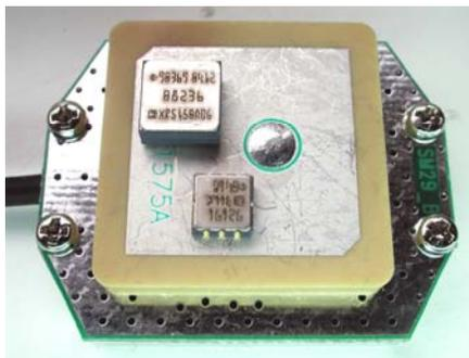
Figure 2 – GPS patch antenna with MEMS yaw-rate linear acceleration sensors.
