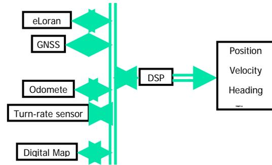
Figure 5 – Basic car navigation concept.
