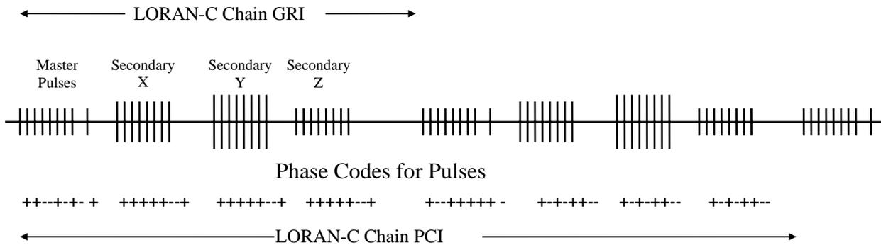
Figure 1. LORAN-C Pulse Architecture
