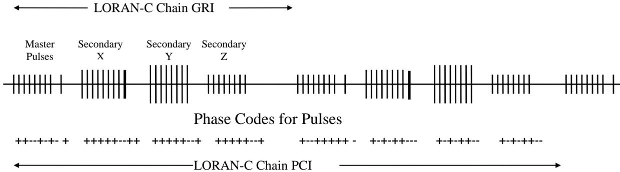
Figure 3. Loran Pulse Architecture with Ninth Pulse Modulation
