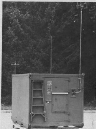
The TACMET shelter is of standard military size and transportable by 2 1/2 ton trucks. Clearly visible are some of the extended weather sensors mounted on the shelter's roof. probe, the Microsonde™. Established in 1963 Beukers Laboratories, Inc. is specialized in design and construction of meteorological, navigational and environmental data acquisition and processing systems. □
