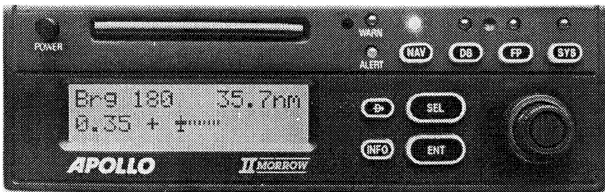
Aircraft loran displaying bearing and distance to waypoint. The second line shows the magnitude (0.35NM) and direction of the XTE. (Photograph courtesy of II Morrow Inc.)
