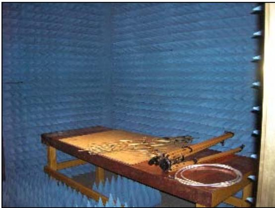
Figure 5: Anechoic chamber, FAATC hangar.
