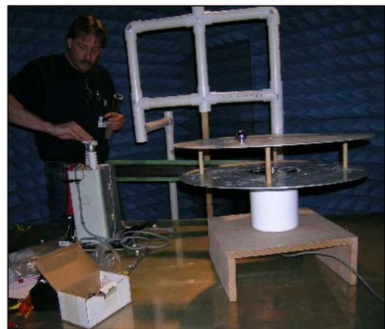
Figure 7: FAATC's Scott Shollenberger prepares the high voltage power supply to calibrate the field mill (right).
