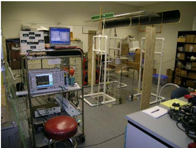
Figure 9: Laboratory with high-voltage equipment installed. Wing section with ion flood and collectors is visible at right, isolated by non-conducting supports. High-voltage power supply is out of sight behind the instrument cart. Note the peripheral ground wire which limits charging of room contents.
