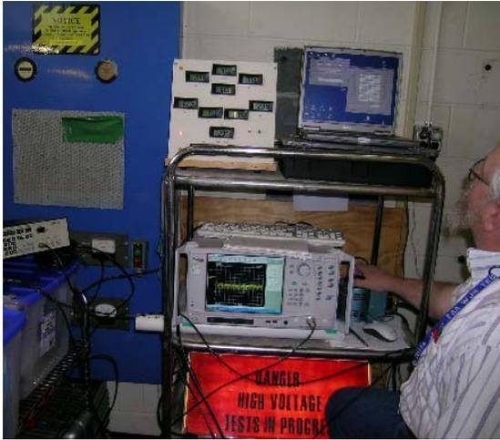
Figure 8: Outside the anechoic chamber, FAA Technical Monitor Robert Erikson sets up the high-voltage monitor panel, PC for data recording and the spectrum analyzer.
