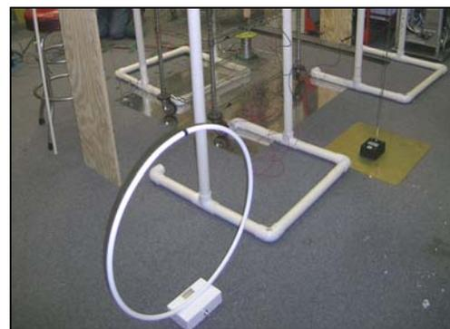
Figure 22: Standard h-field and e-field antennas
