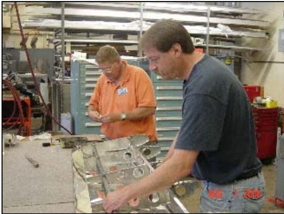
Figure 4: FAATC's John Tatham and Scott Shollenberger fabricate the wing section for high-voltage experimentation.
