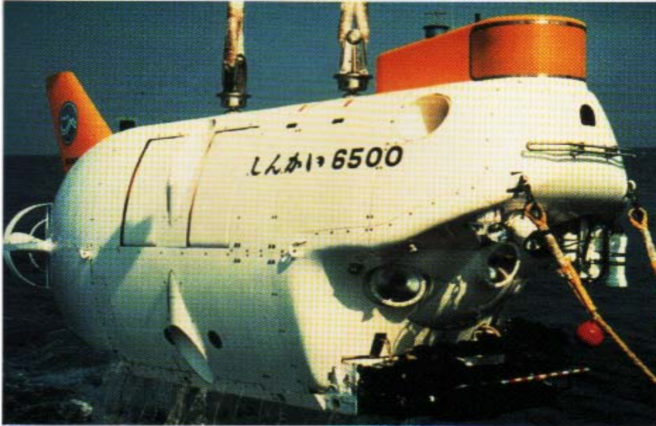
The Shinkai 6500 of JAMSTEC is a manned research submersible constructed in 1990 for operational depth to 6500m. It has a length of 9.5 m, a width of 2.7 m, a height of 3.2 m and a weight of 26 t. Its pressure hull is 2.0 m in diameter and
