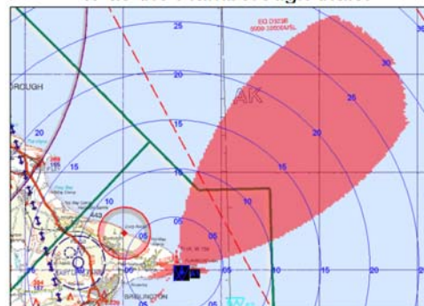
Figure 4: Jamming Zone During Trials Conducted by the General Lighthouse Authorities (GLA) of the U.K. and Ireland (Last, 2010). These are referred to as the Flamborough trials.
